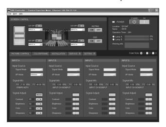
Click any of the PICTURE CONTROL, COLOR/ FRAME and INSTALLATION buttons to display the desired control window.
